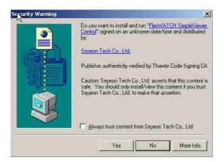
When the Client pc is not connected to Internet, you need to manually install ActiveX components in your viewing PC.
